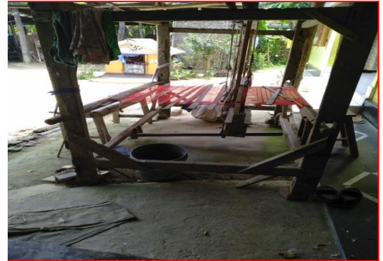
Khadi weaving loom of poor artisan need immediate replacement Photo on 10-07-2018
